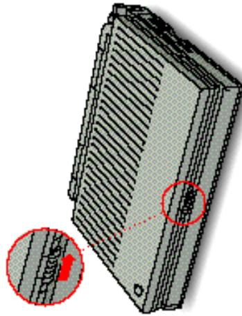
3. Raise the display to a comfortable viewing angle.
