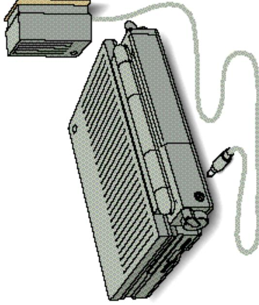
2. **Plug the power adapter cable into the power adapter port on the computer's back panel.**
