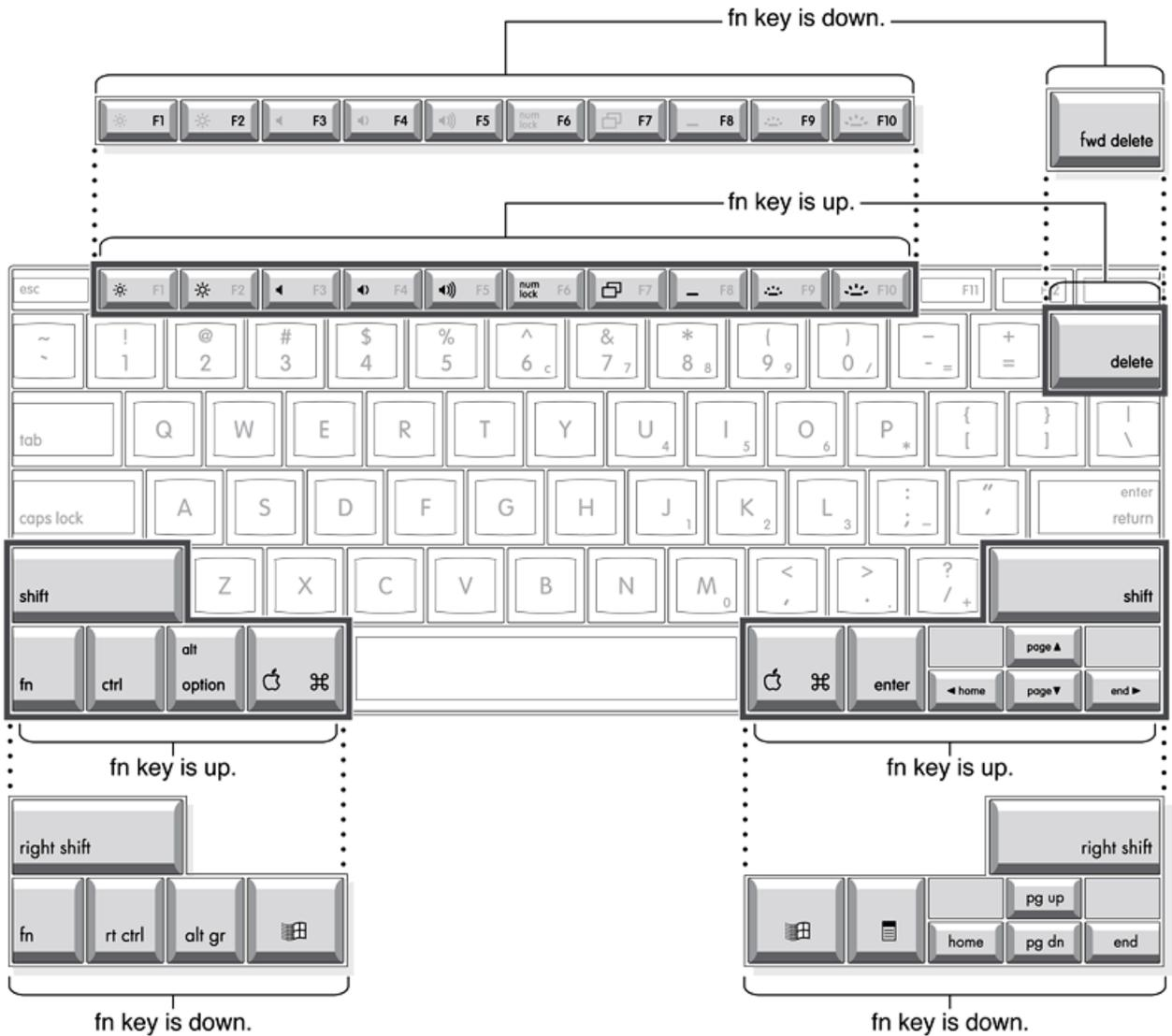
Figure 3-8 Embedded numeric keypad operation
