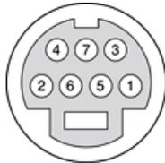
**Table 3-17** Pin assignments for the S-video output connector
