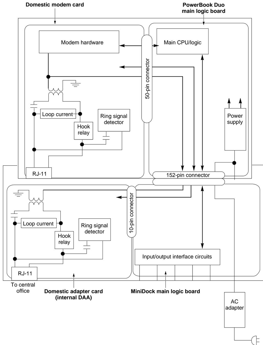
**Figure 5-7** Interface between modem card and the Duo Dock
