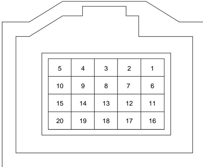
**Table 11-4** Floppy disk drive connector signal assignments
