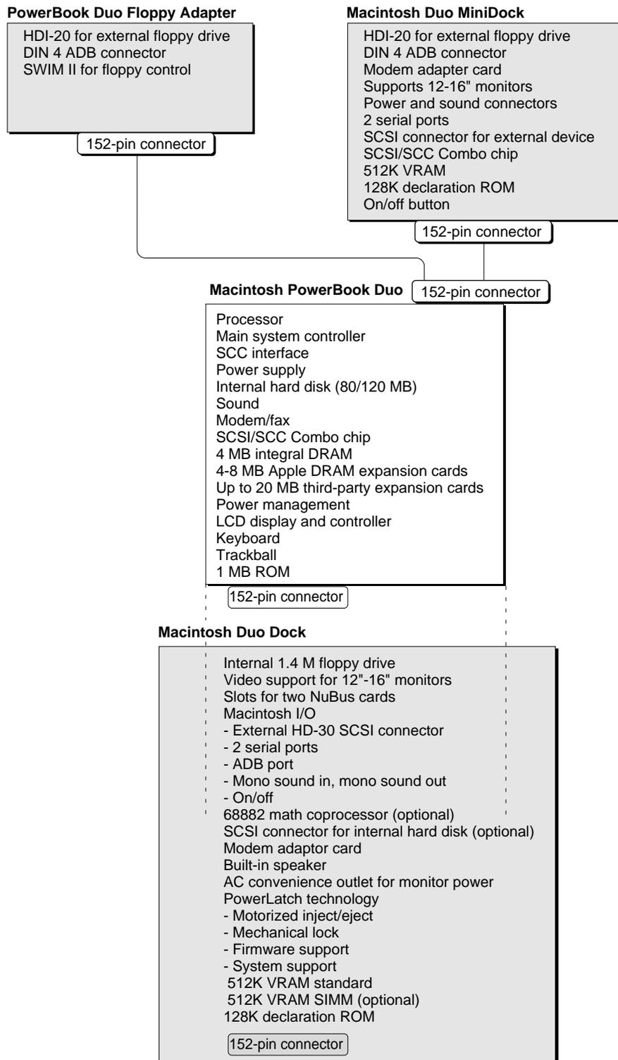
**Figure 1-3** PowerBook Duo simplified block diagram
