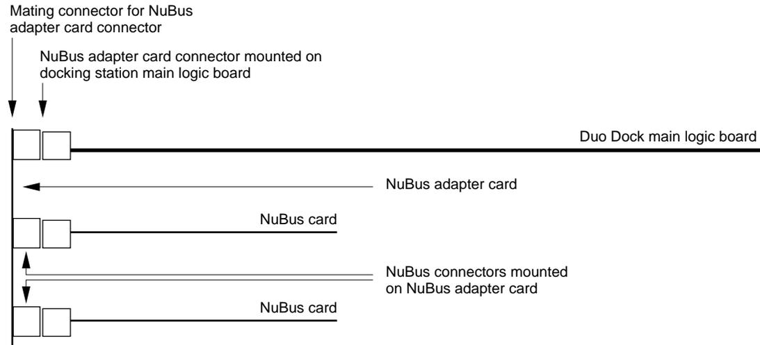
**Figure 14-14** Front view of NuBus adapter card showing connectors
