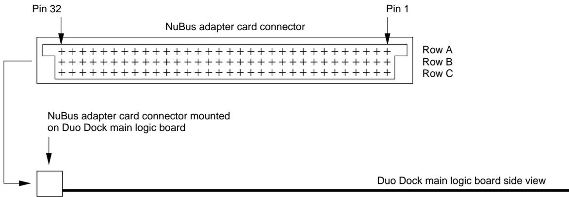
**Figure 14-13** NuBus adapter card mounting configuration
