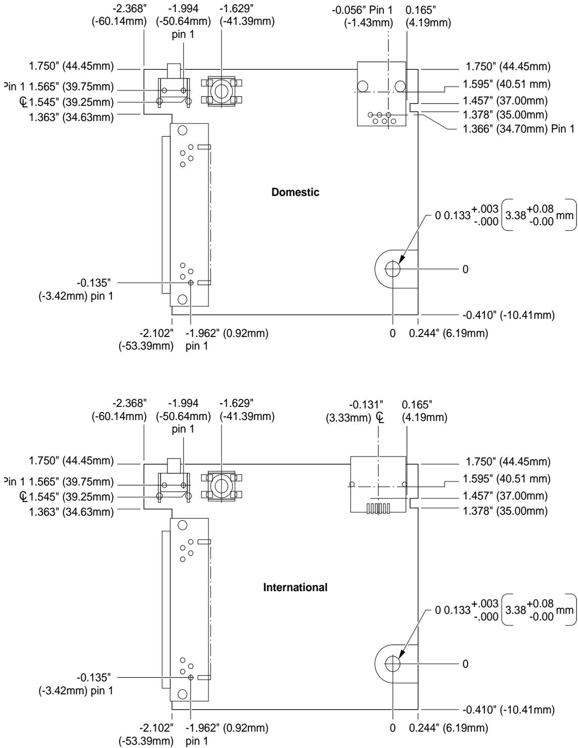
**Figure 5-3** Modem card component height
